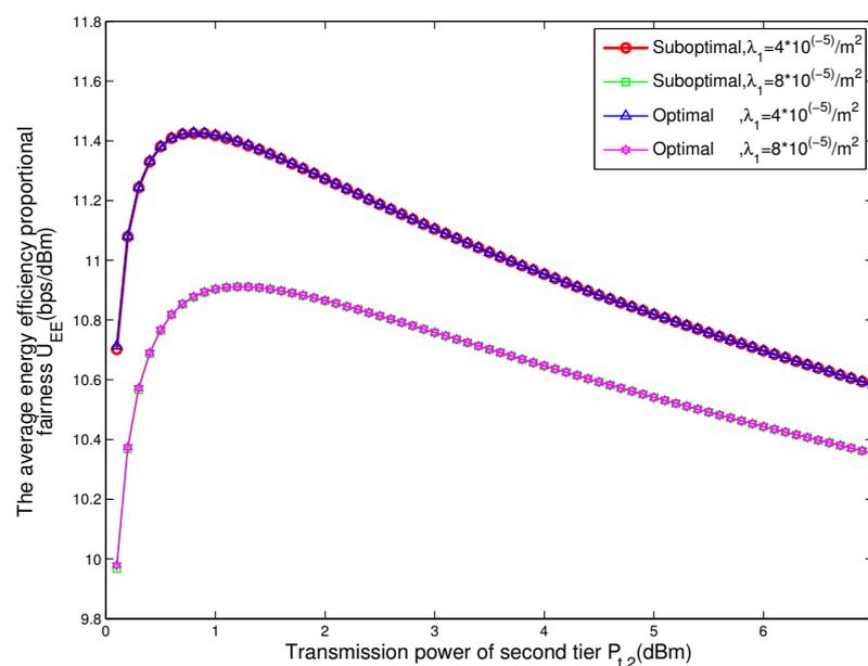
**Figure 4.** The mean energy efficiency proportional fairness with respect to the association probability of tier 2 obtained from the proposed suboptimal scheme and optimal two-dimension search scheme for different values of the transmit power of base stations (BSs).
