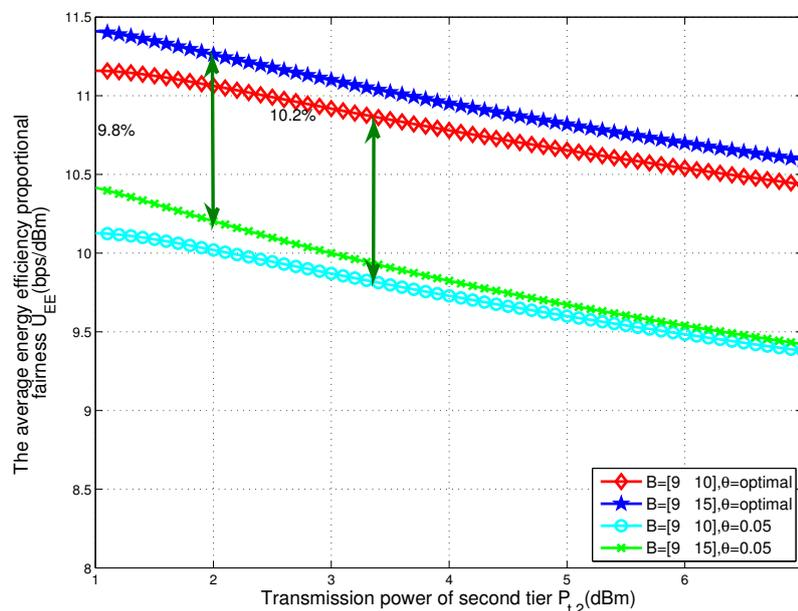
**Figure 3.** Energy efficiency proportional fairness of total two-tier heterogeneous WPCNs with respect to the transmit power of BSs in tier 2 for different values of the tier-2 cell association bias  $B_2$ .
