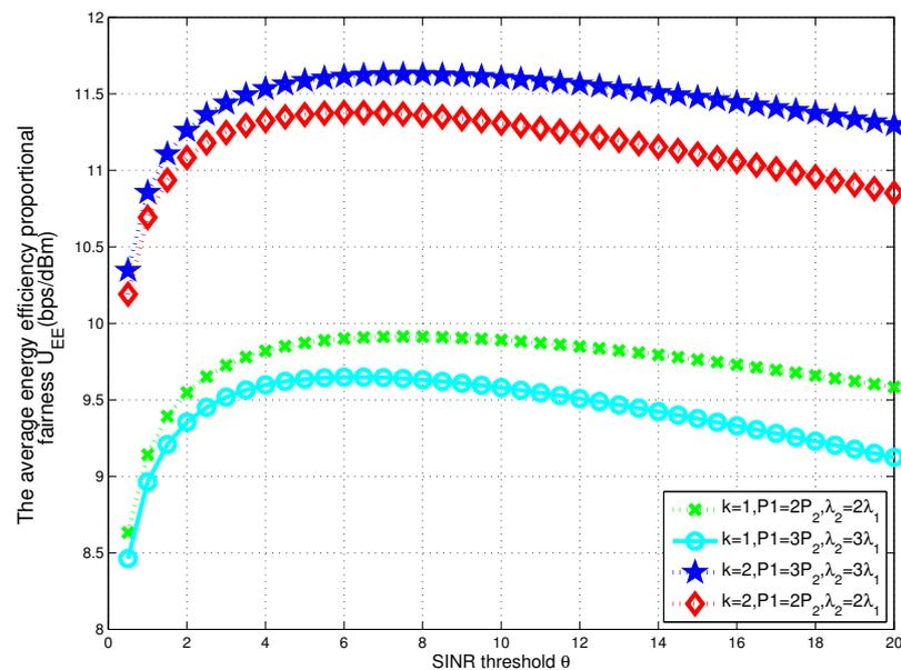
**Figure 2.** The relationship between energy efficiency proportional fairness utility function and the receive threshold for different transmit powers and densities of BSs in two-tier heterogeneous WPCNs.
