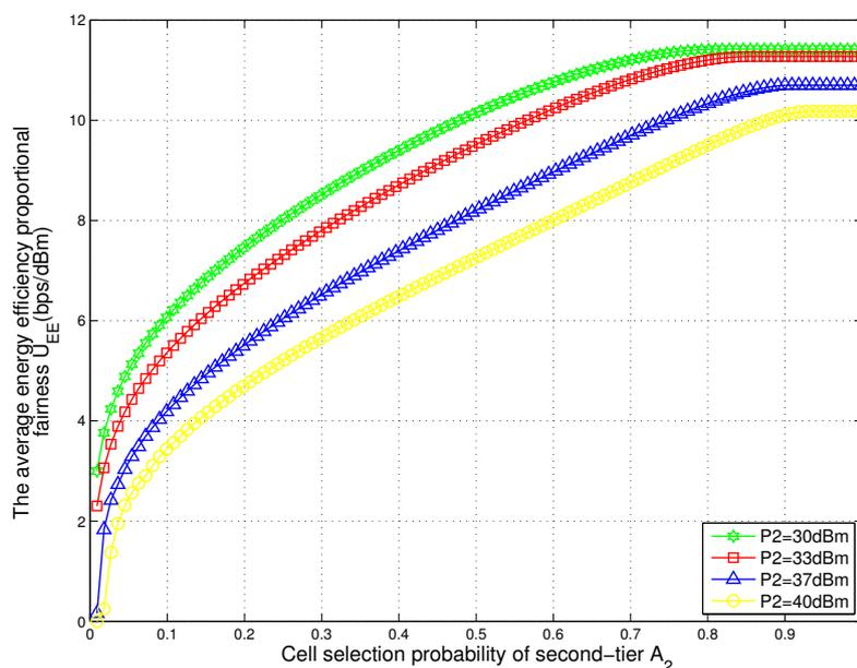
**Figure 6.** The energy efficiency proportional fairness of total two-tier heterogeneous WPCNs with respect to the association probability of tier 2 for different values of the transmit power of BSs.
