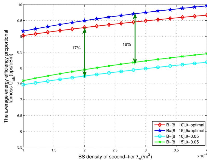
**Figure 5.** The energy efficiency proportional fairness of total two-tier heterogeneous WPCNs with respect to the density of BSs in tier 2 for different values of the tier-2 cell association bias  $B_2$ .
