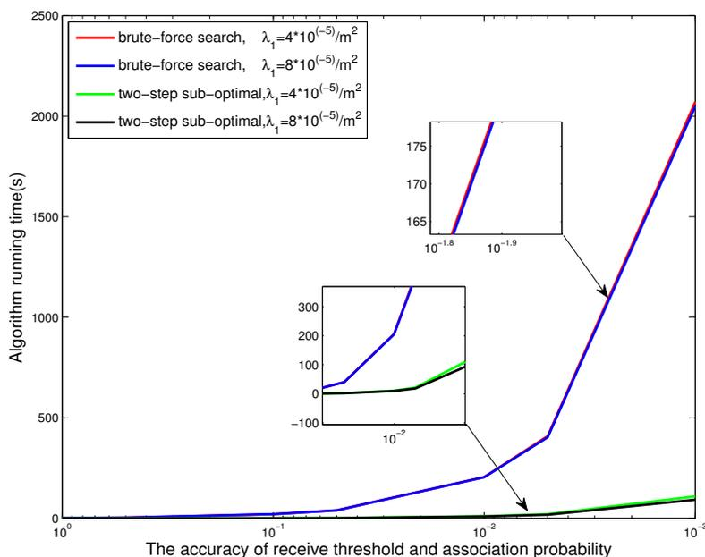
**Figure 7.** The time cost of brute-force two-dimensional search algorithm and two-step sub-optimal algorithm with respect to the accuracy of system parameters.
