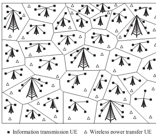
**Figure 1.** System model of a multi-tier heterogeneous wireless powered communication network (WPCN).
