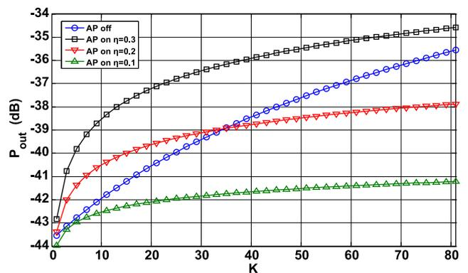
**Fig. 4** Impact of femtocell users number on the macrocell user outage probability in TTCANs
