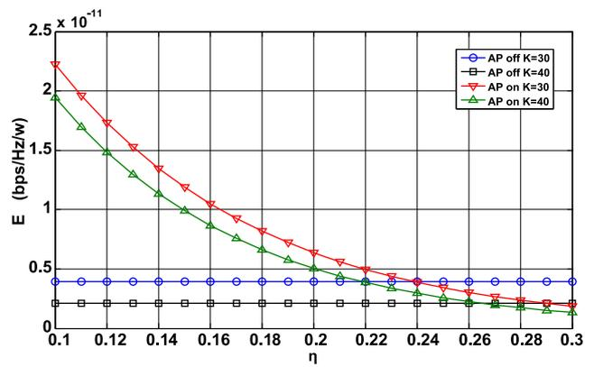
**Fig. 3** Impact of the ratio of the required uplink transmission power in a macrocell over the required uplink transmission power in a femtocell on uplink energy efficiency of TTCANs
