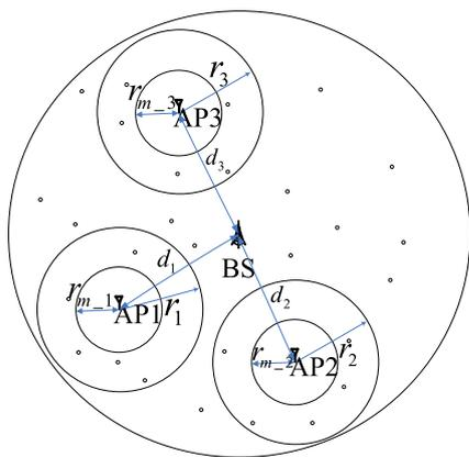
**Fig. 1** System structure of a wireless TTCAN
