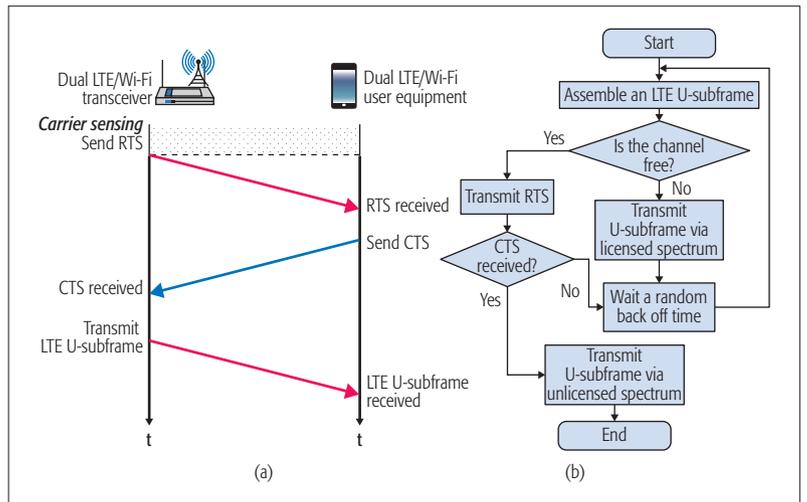
FIGURE 2. The proposed a) MAC protocol diagram; b) transmission algorithm for S-CASLUA.
