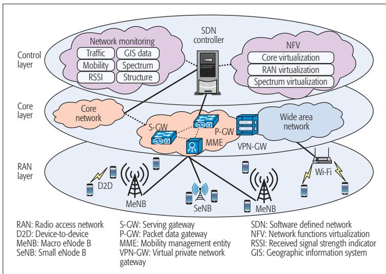
FIGURE 1. Simplified architecture of heterogeneous mobile networking based on SDN and NFV.
