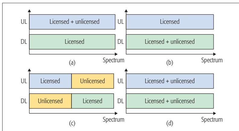
FIGURE 4. Four spectrum-sharing strategies for uplink and downlink channels.
