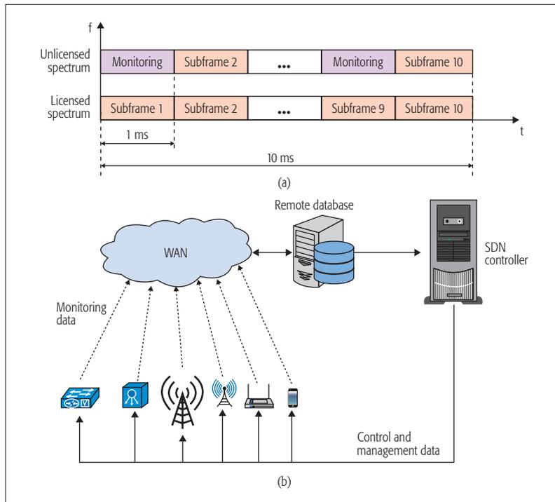
FIGURE 3. a) Dual-frame structure and b) simplified architecture of SDN-CASLUA.
