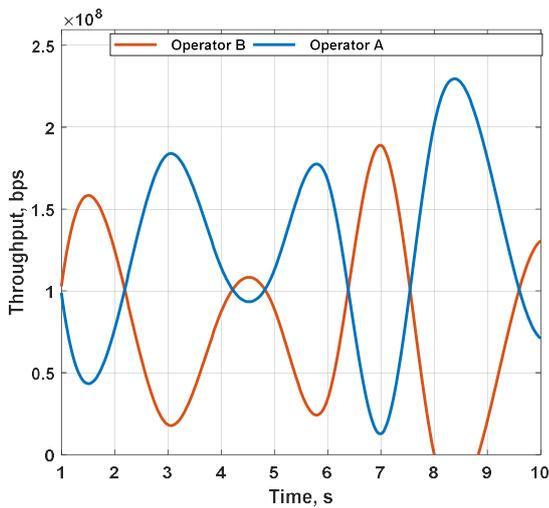
Fig. 2. Throughput in case of random spectrum sharing between two operators in unlicensed spectrum.
