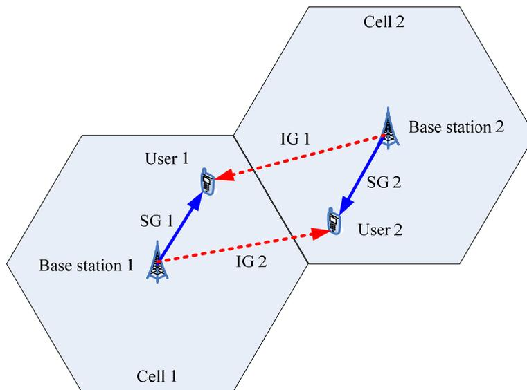
**Fig. 2.** Two-cell cellular network system model
