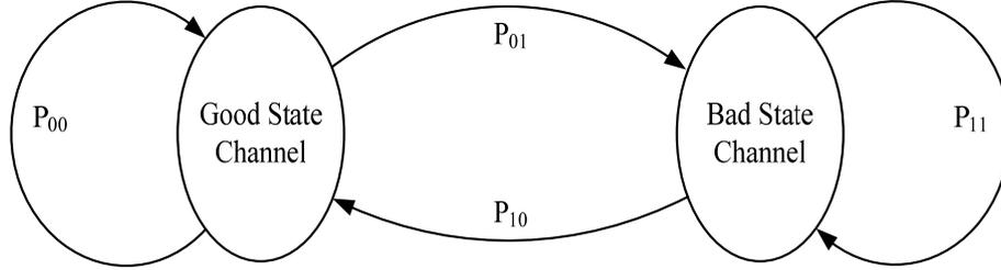
**Fig. 5.** State transition diagram of two-state Markovian wireless channel
