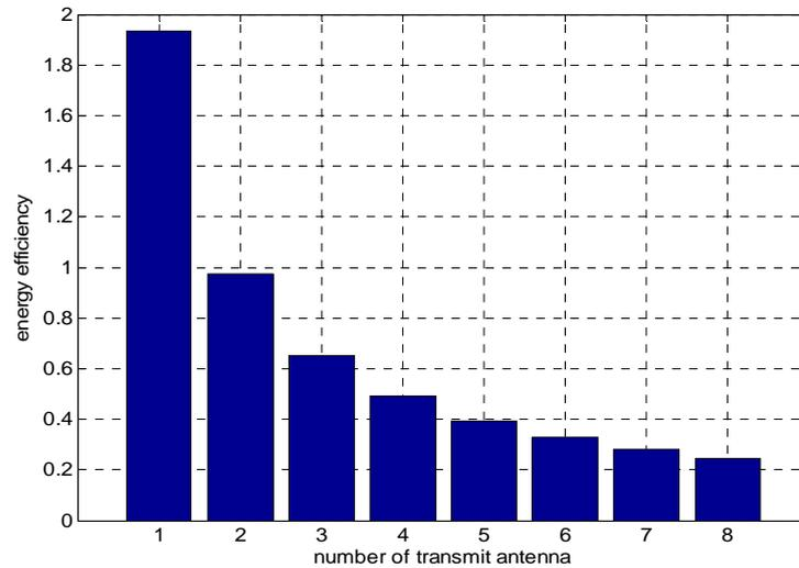
**Fig. 6.** Impact of number of antennas on energy efficiency
