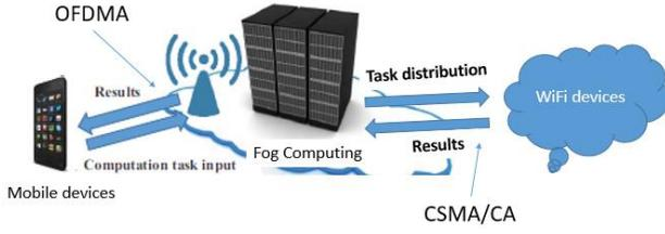
Figure 1. Fog computing system with WiFi network
